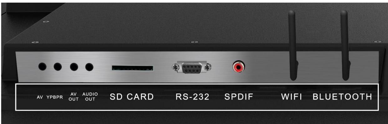
Figure 4 Rear Inputs (Side)
