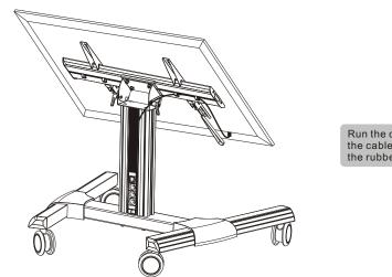
Run the cables through the cable clamps and the rubber strip.
