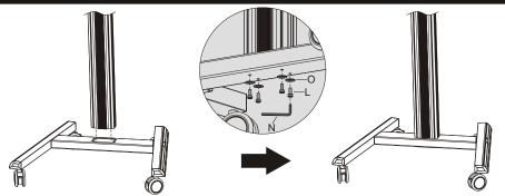
Attach the column to the assembled base using the appropriate screws and washers. Tighten all screws with an Allen key. **NOTE:** Lock the brakes on the casters to avoid any sudden movements during installation.
