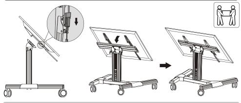
Lift the display carefully and pull downward two straps at the same time , then hook the adapter brackets to the universal plate. Fasten the adapter brackets to the universal plate by releasing the straps.
