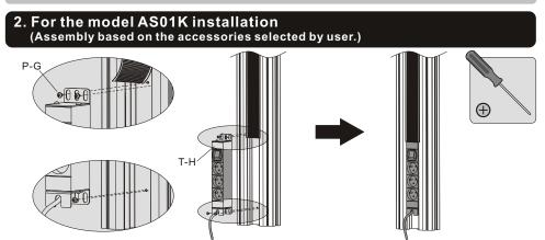
Attach the power socket to the back of column using the appropriate screws. Tighten all screws with a phillips screwdriver.
