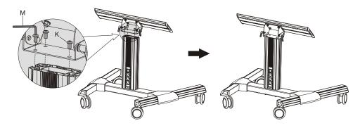
Attach the universal plate to the column using the appropriate screws. Tighten all screws with an Allen key.
